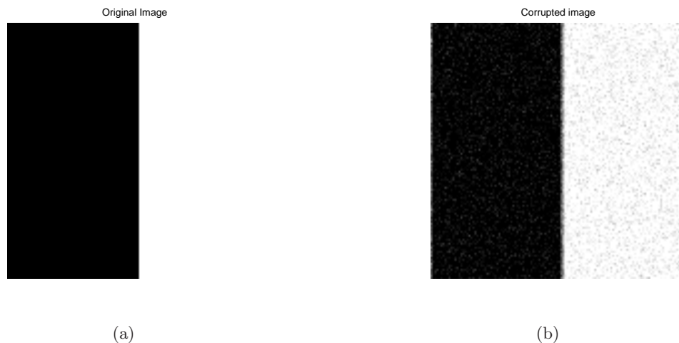
Figure 6.9. (a) Original image that is black on its left and white on its right side. (b) Image corrupted by a blur operator with averaging kernel supported on 3 \times 3 pixels and uniform values 1/9 and additive white Gaussian noise with variance 20.
