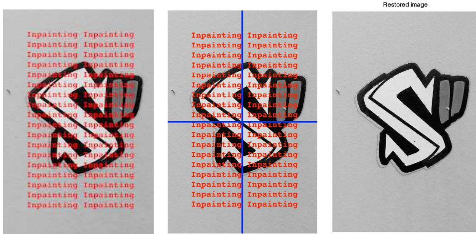
Figure 4.21: Inpainting with the parallel domain decomposition strategy (4.40): (l.) the vandalized image of size 1768 \times 2656 pixels; (m.) its decomposition into four domains; (r.) the restored image computed with (4.40)
