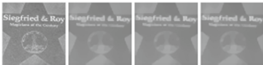
Fig. 2 From left to right: 64x64 pixel input image g and respective denoised outputs for semi-implicit, semi-implicit accelerated and semi-smooth Newton algorithms
